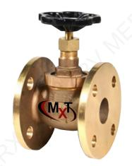
Bronze MXT globe valves with bronze disc and seat, pressure rating PN 16, straight pattern, flat faced flanges ace. to DIN PN 16, screwed and secured bonnet, inside screwed stem and rising handwheel. Primary application area is aboard ships where a light bronze construction is desirable.
